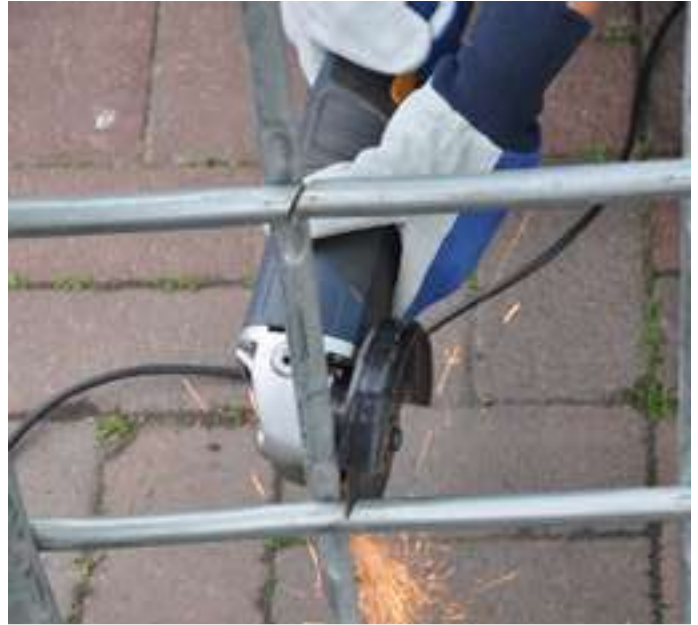
Cut the frame at the required height for your growbed
