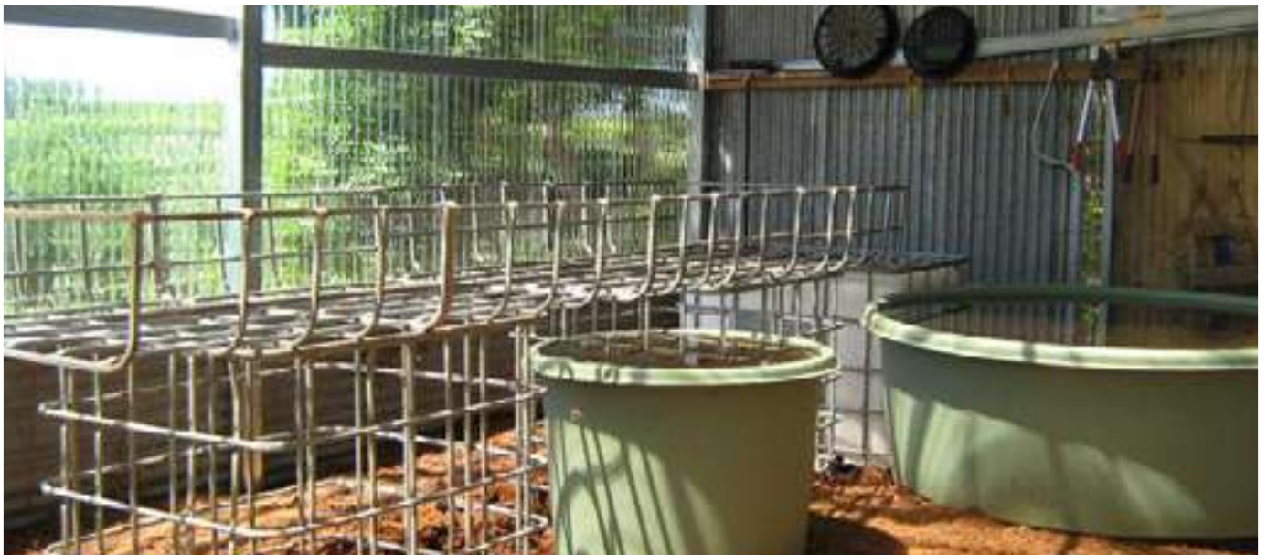
Rather than the conventional way most people cut and mount their IBC beds, Tristrin cuts them in a different way which adds more support to the base of the growbed
