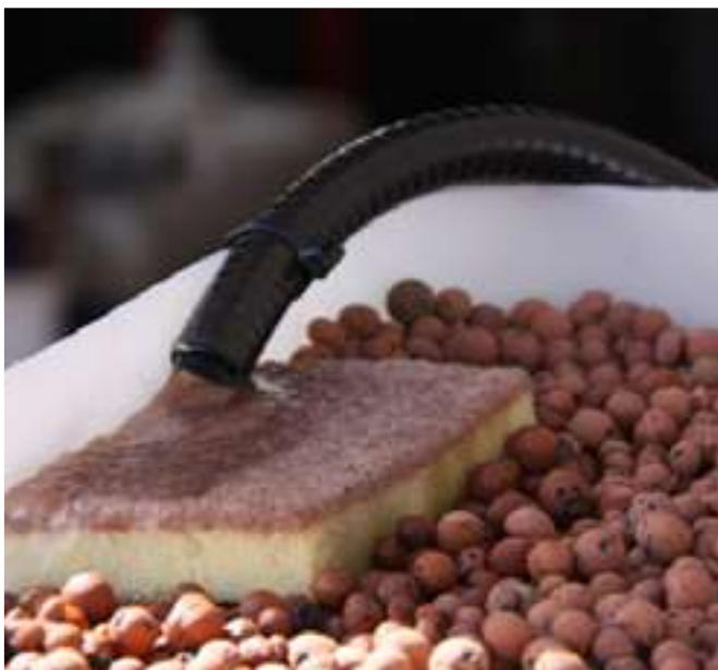
Water entering growbed through filter pad
