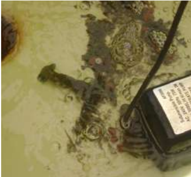
3000lph submersible pump
