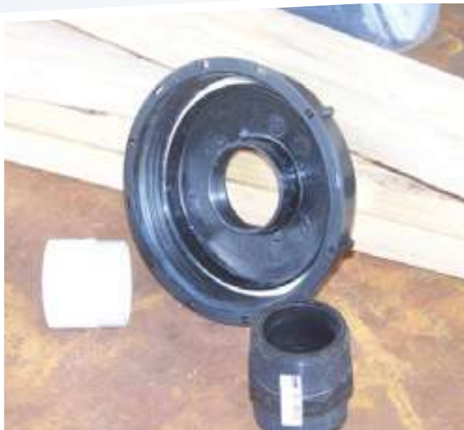
2 inch thread on lid makes for easy adaption
