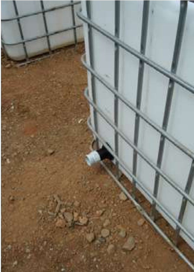
Tank fittings are one of the safest ways to plumb an IBC
