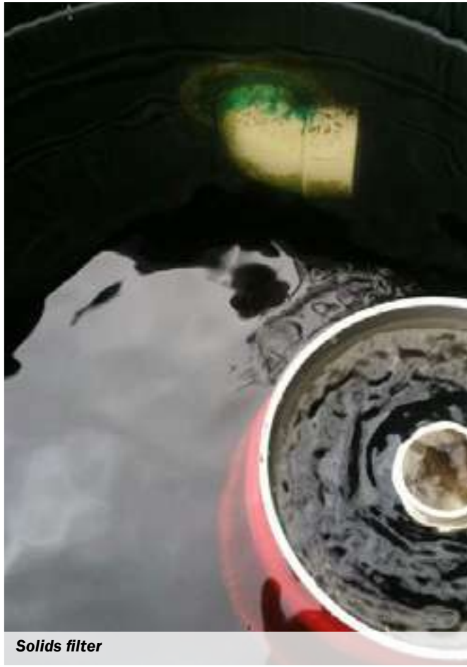
The fish tanks and barra bed drains tee into the trout bed drain and go into the filter
