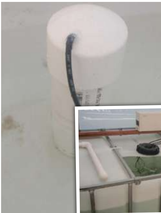
Two different siphons were tried, one bell siphon with a breather hose
