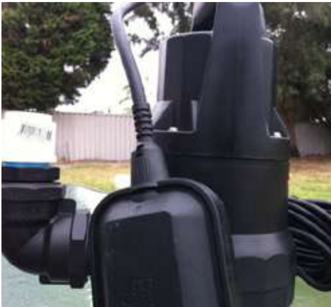
Pump with float switch
