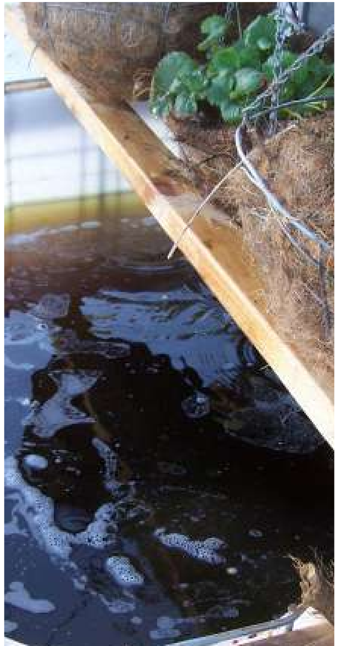
Water flows through the coconut fibre and coir turning the water brown
