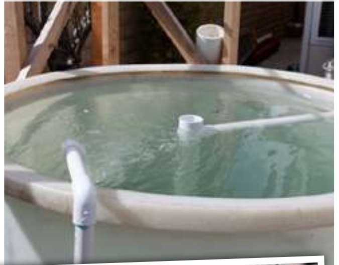
The fish tank with SLO (solids lift over flow)
