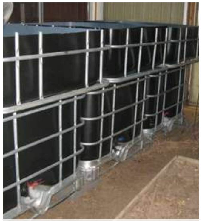
Bases were spray painted to reduce light and stop algae growing
