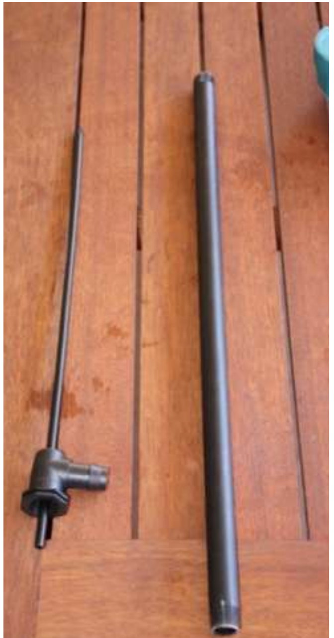
Venturi, all made from reticulation parts
